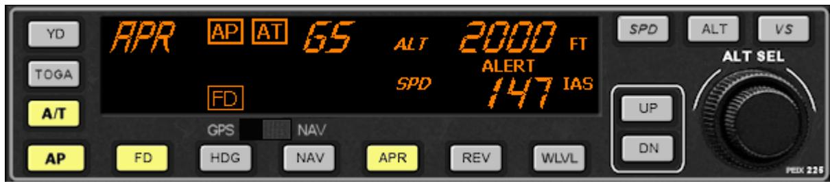
The same performed with Boeing 737 (or any aircraft with an Auto-throttle). With Auto-throttle and Flight director on and showing the selected approach speed. Remember, without an auto-throttle, as PiC you are responsible for managing the throttle to ensure efficient capture of the glideslope !
