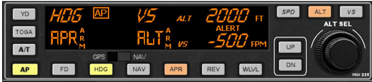
The plane is following the heading selected on the instrument's heading bug, APR is armed waiting to capture the ILS localizer, and ALT is armed because the plane is descending (and it follows the Vertical Speed). Alert appears due to current alt (2500ft ) and selected alt (2000 ft) is less than 1000 ft to reach.
