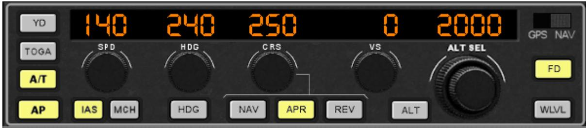
The illumination of the buttons is explained above (previous pages). Essentially there are three types of illumination: Off, Armed and Active - Active = yellow; Armed = orange.
