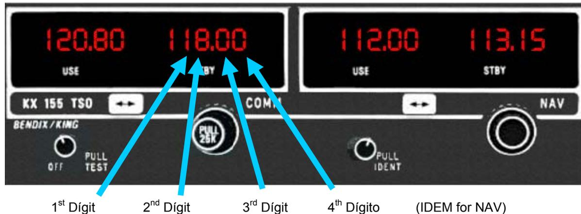
**Example:** To insert the freq 123.45 in STBY of COM 1, press: **C2345**
